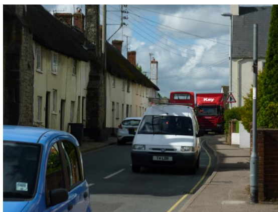
School St (east side) – HGV inc. mirrors are 3m wide, so not enough room for commercial vehicles to pass oncoming traffic
